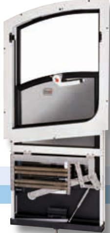
Bulkhead door, with maintenance and advertising-space cover, Bombardier (outside view)
