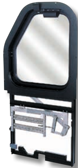
Spring-assisted drop window Bombardier
